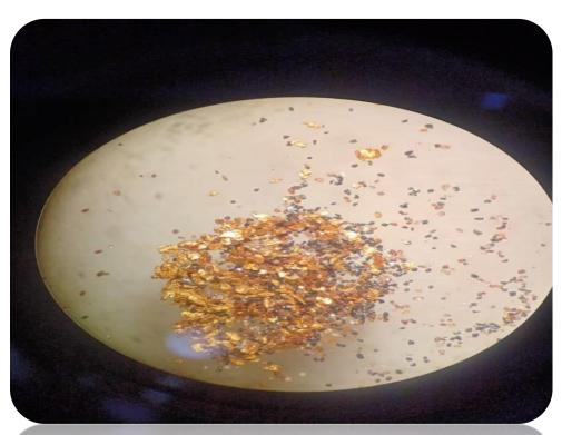
Magnification Stereo microscope use to visualize invisible gold specs and to study the shape and size of gold grains.
